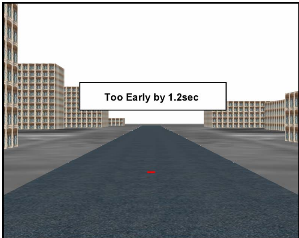
Figure 1: Example of a landing simulation display used in the current study with both lexical and pictorial feedback on the accuracy of flare timing.
